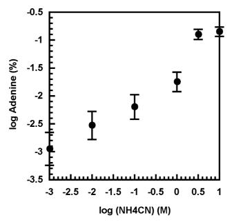
*Figure 3.* Adenine yield from the unhydrolyzed supernatant as a function of  $NH_4CN$  concentration at 80 °C after 16 days.
