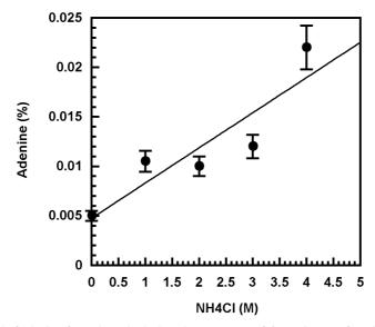
*Figure 4.* Yield of adenine from the unhydrolyzed supernatant of 6 m HCN as a function of ammonia concentration at 80  $^{\circ}$ C after 11 days.
