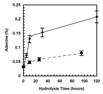
*Figure 6.* Adenine yield from the supernatant from an 80 °C 10 M NH<sub>4</sub>CN polymerization conducted for 48 hr as a function of hydrolysis time in 0.1 M pH 8 phosphate at 120° (circles) or 140 °C (diamonds).
