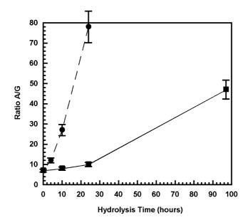
*Figure 9.* Ratio of adenine to guanine produced from the 6 N HCl hydrolysis of the supernatant of a 10 M NH<sub>4</sub>CN polymerization conducted at 80  $^{\circ}$ C for 48 hr.
